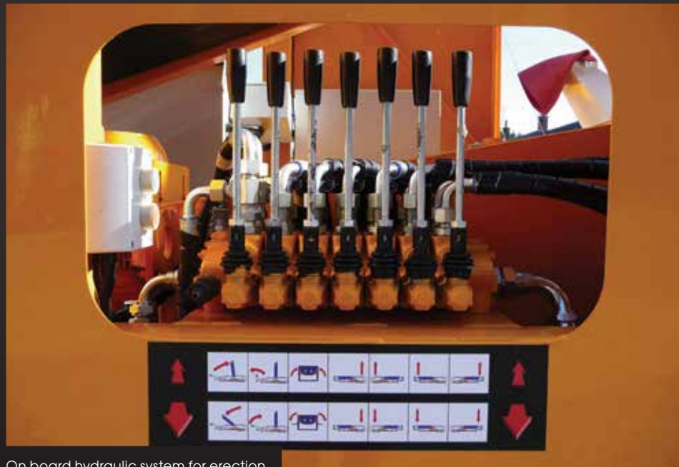
On board hydraulic system for erection
